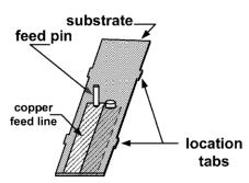
perspective view of the pcb support structure
